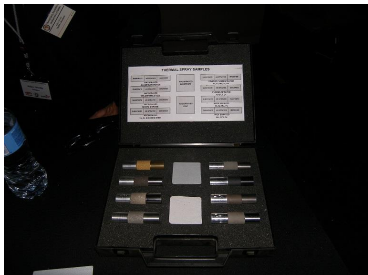
Adam Wintle of the Thermal Spray Association of Southern Africa with a selection of metal coupons treated with different metal thermal spray applications
