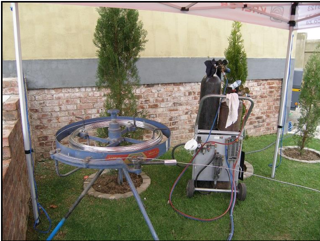
Above: Zinc coil feeder and carrier gas setup
